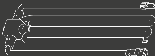
Power supply Y connection cable 1.5m (L-CAB-Y-1.5)
